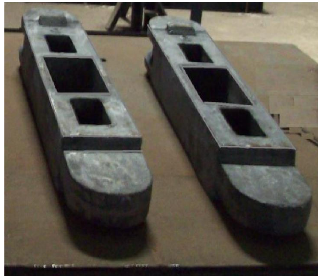
CASTING CHAIN LINK SPEC: IS3038 GD 4
