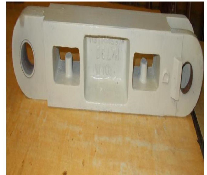
CASTING CHAIN LINK AFTER MACHINING
